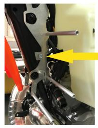
TURN ONLY THE NUT AND POSITION THE BRACKETS BEFORE TIGHTENING (FIG. A, B, C, D, E)
