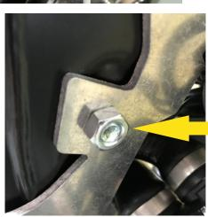
AFTER SETTING THE BRACKETS, TIGHTEN THE NUT. THE SCREW IS TO BE ALIGN WITH A NUT.
