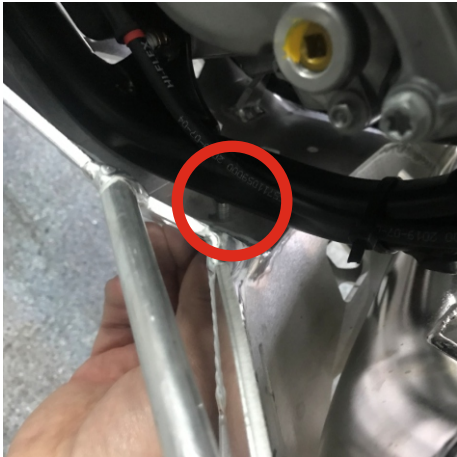
GRIP SCREWS TO FRAME SOCKETS
