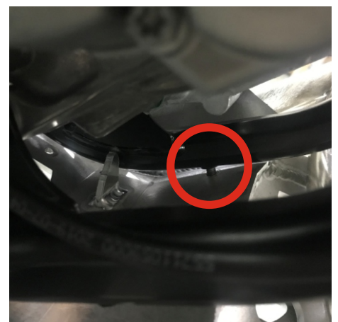
GRIP SCREWS TO FRAME SOCKETS
